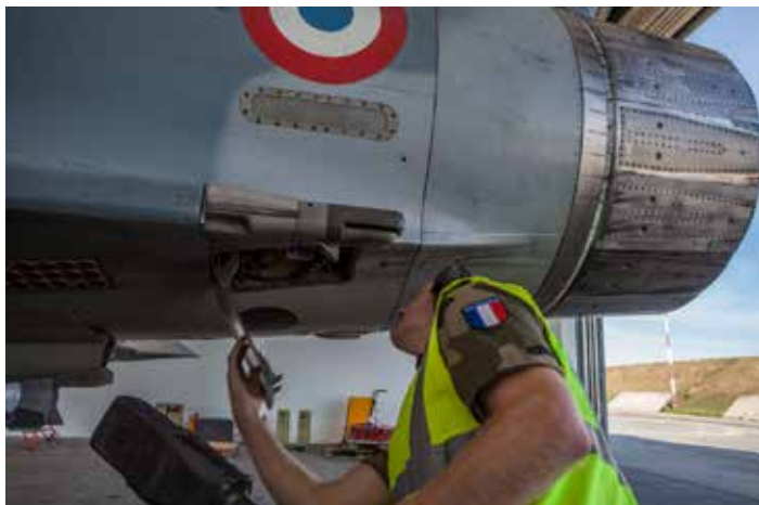
Sergeant Chef Jeremy disconnecting the external power unit from a Mirage 2000C fighter jet in order to prepare the take-off.
