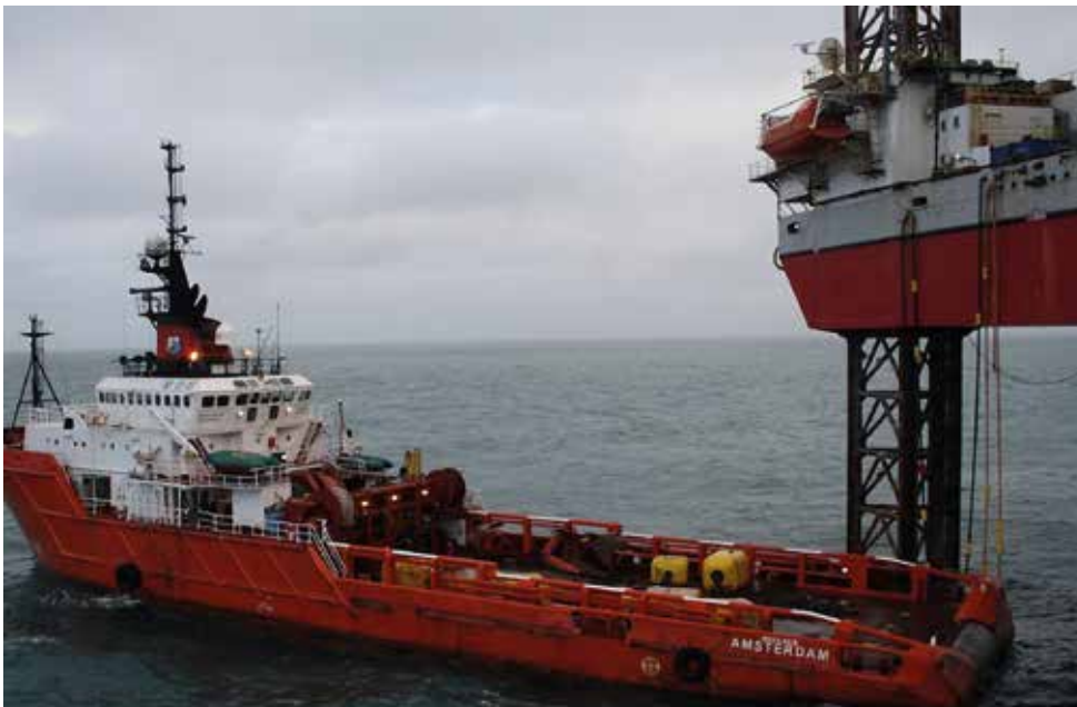
AHTS 'Boulder': The Boulder, an Anchor Handling Tug Supplier with 12,000-horse power can accurately manoeuvre between the legs of an oil rig.
